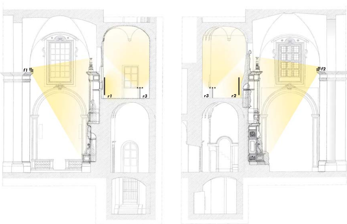
r1 r2 r3 雕塑组后方唱经楼，f50灯具分布 choir behind the sculpture ensemble, f50 light fittings distribution
